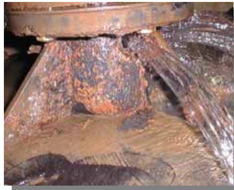
▲Degraded part of air valve
