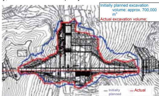
Initially planned and actual extents of excavation
