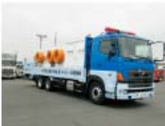
Pump truck (Pumping capacity 60,000 l/min.)
