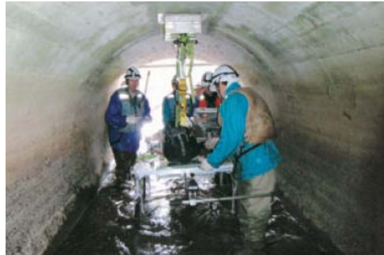
Use of the radar exploration to check the back void of concrete lining in the water tunnel
