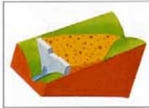
Sediment has been trapped to capacity.
