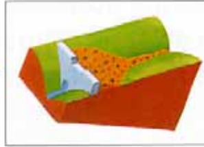
Trapped sediment has been gradually carried downstream.
