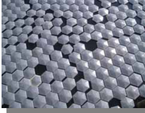
▲Hexagon float used for restraint of algae or water bloom
